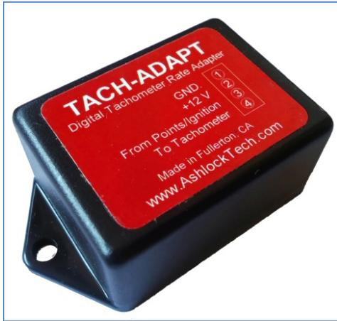
*Avoid replacement or rebuild of your stock or vintage tachometer. Instead, use TACH-ADAPT to properly drive your old tach from the new engine or ignition system you converted to.*
